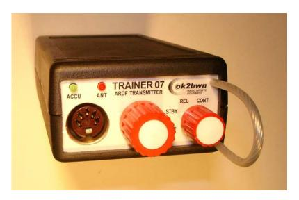
The operation is very easy: just install the antenna, plug in the connector and transmitter automatically recognizes the proper band and starts operation.
