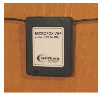
This transmitter was especially designed for training purpose, foxoring competitions, promotion events and other special ARDF events. Frequency, transmitted code, keying speed and timing schedule are widely adjustable. Integrated antenna make the installation very easy – just hang it at a tree branch.
