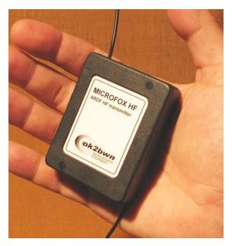
This transmitter was especially designed for training purpose, foxoring competitions, promotion events and other special ARDF events. Frequency, transmitted code, keying speed and timing schedule are widely adjustable. Integrated antenna make the installation very easy – just hang it at a tree branch.
