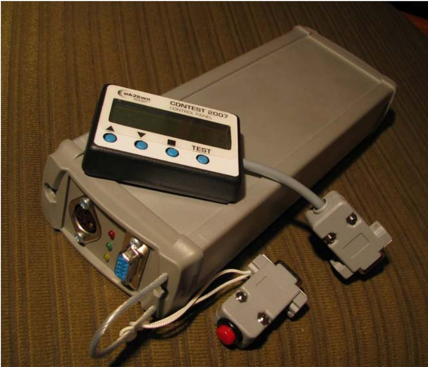
**After all parameters are set, the operation is very easy: just install the antenna, plug in the connector and transmitter automatically recognizes the proper band and starts operation. Just one button click and internal automatic antenna tuner will provide optimum matching of the HF antenna.**
