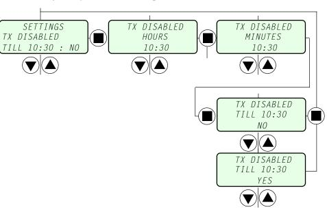
The time at which the transmitter shall commence operation, can be set to any time up to 24 hours in the future.
