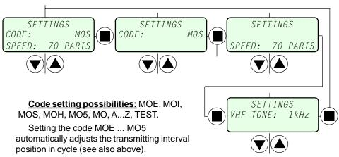
**NOTE: DO NOT USE THE TEST CODE!** The TEST code is intended only for testing and diagnostic purpose. At this setting transmitter generates a continuous carrier, which is allowed only for a short time and into the defined load.
