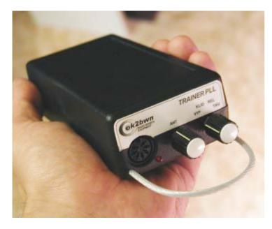
The TRAINER PLL ARDF transmitter is designed for local and regional ARDF competitions and training of any level. The possibility of frequency, transmitted code, keying speed and timing schedule adjustments opens the new area in the ARDF competitions and allows using more transmitters on different frequencies.
