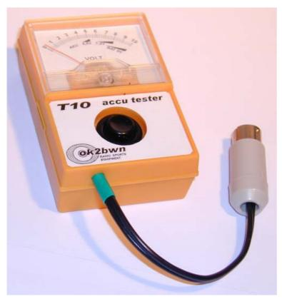
T10 tester is designed for accumulator status check of ARDF receivers of COMPACT and SUPERFOX series (and other similar types as well). It is a useful tool, necessary for the proper treatment of NiCad accumulators.
