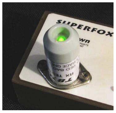
The T810 tester is the sophisticated, microprocessor controlled device designed for accumulator status check of ARDF receivers of COMPACT and SUPERFOX series (and other similar types as well).
