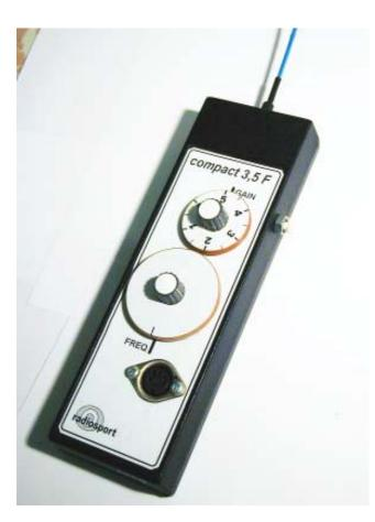
The COMPACT 3,5 F receiver is designed for the wide company of competitors including beginners. Its ergonomical solution results from the following features: low weight and small size, all receiver controllable by single hand even in full run, shock-resistant, waterproof house and low price.
