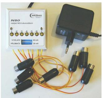
2. The N80 charger is designed for charging 7 ARDF receivers of COMPACT and SUPERFOX series or transmitters of TRAINER and COMPACT TX series. The charging current can be adjusted independently for each output at 28 or 80 mA. Charging status is indicated by a LED diode.
