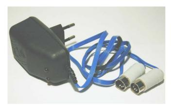
1. The N28 charger is designed for charging all ARDF receivers of COMPACT and SUPERFOX series. One charger can handle any two receivers. The charging current is stabilized at 28 mA. Charging status is indicated by a LED diode.
