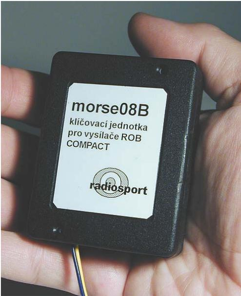
*This unit is designed for connecting to the COMPACT series ARDF transmitters. It brings significant improvement of code and timing options of the transmitters, useful for training purposes, foxoring competitions and promotion events.*
