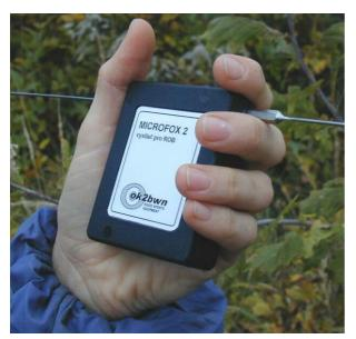
This transmitter was especially designed for training purpose, foxoring competitions, promotion events and other special ARDF events. Transmitting code, keying speed and timing shedule are widely adjustable. Integrated antennas make the installation very easy – just hang it at a tree branch.
