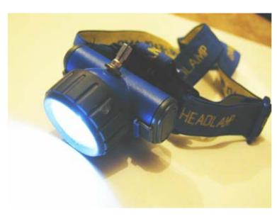
This headlamp is designed for walking, running and other outdoor activities in night. Compared to common headlamps, LEDLAMP2 contains switching DC/DC converter, which provides high efficiency and stable light power within the whole lifetime of the batteries.
