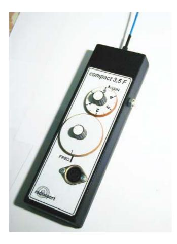
The COMPACT 3,5 F receiver is designed for the wide company of competitors including beginners. Its ergonomical solution results from the following features: low weight and small size, all receiver controllable by single hand even in full run, shock-resistant, waterproof house and low price.
